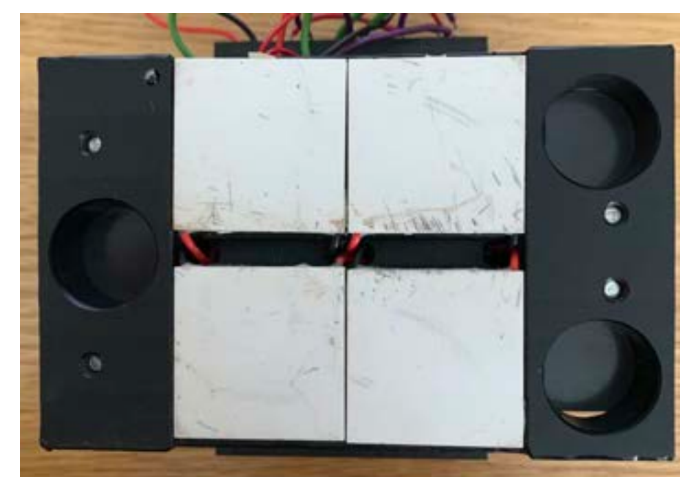
Figure 2. Top view of apparatus showing the four TEGs embedded in the plastic base.
